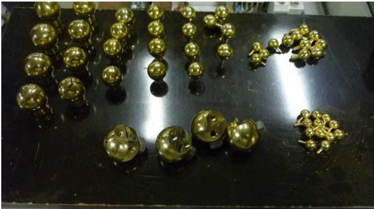
Next came the tedious process of making the brass end balls. I did this manually, but it would be a task for CNC work.
