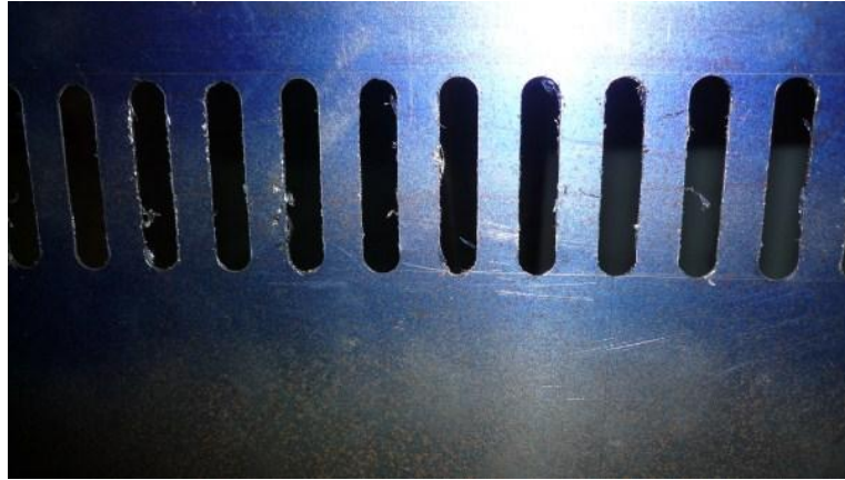
Rough milling before finishing.
