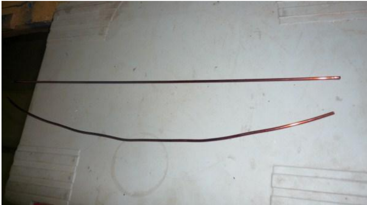
In order to neaten up the enabled copper wire, it was first stretched using a bench vice and a pair of pliers. The straight piece is the end result.
