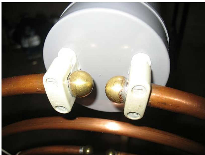
Connection of antennas to the Tesla coils
