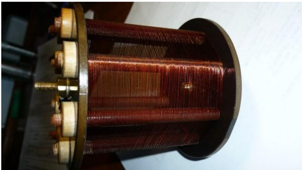
The finished item, sprayed with anti tracking lacquer.
