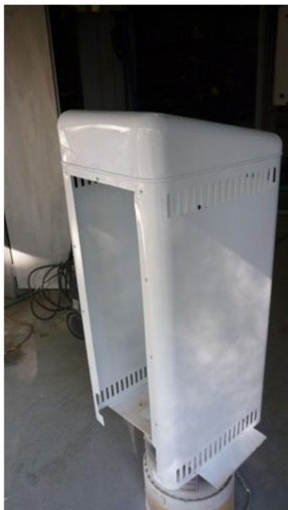
Final coat of white 2K Epoxy paint is applied.
