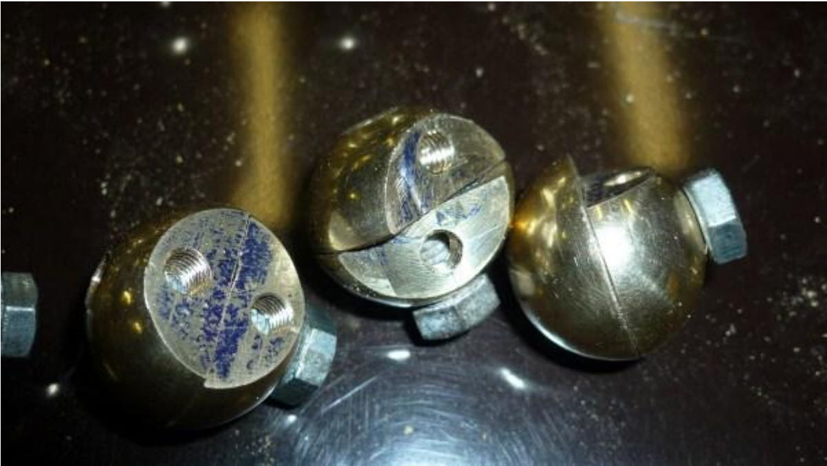
Finished joint knuckles.
