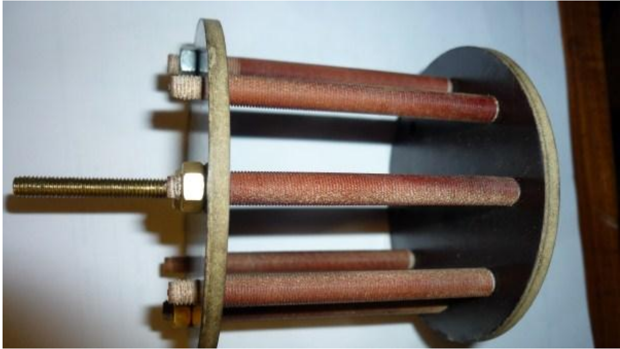
The finished cage, ahead of winding which was done manually in the lathe for support. The wire has to be manually guided in to all the groves
