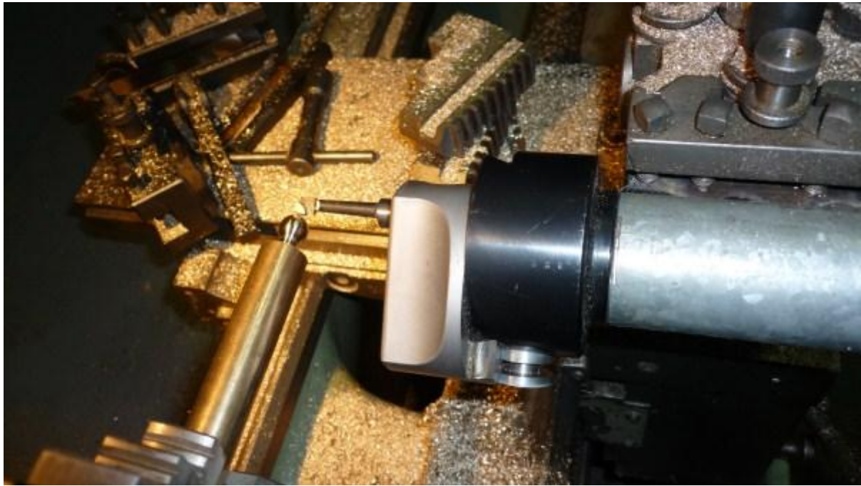
Then using a modification to an adjustable boring bar, and ball making jig was set up.
