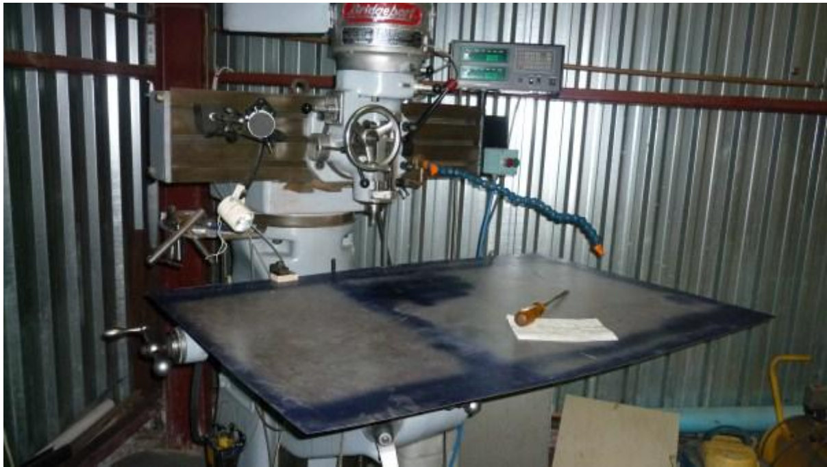
Then the sheet was mounted in the milling machine to mill the cooling slots.
