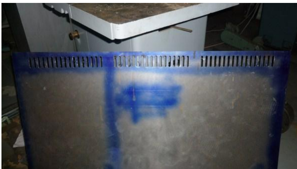
The blank is ready for bending, once the spark gap monitoring hole is cut out.
