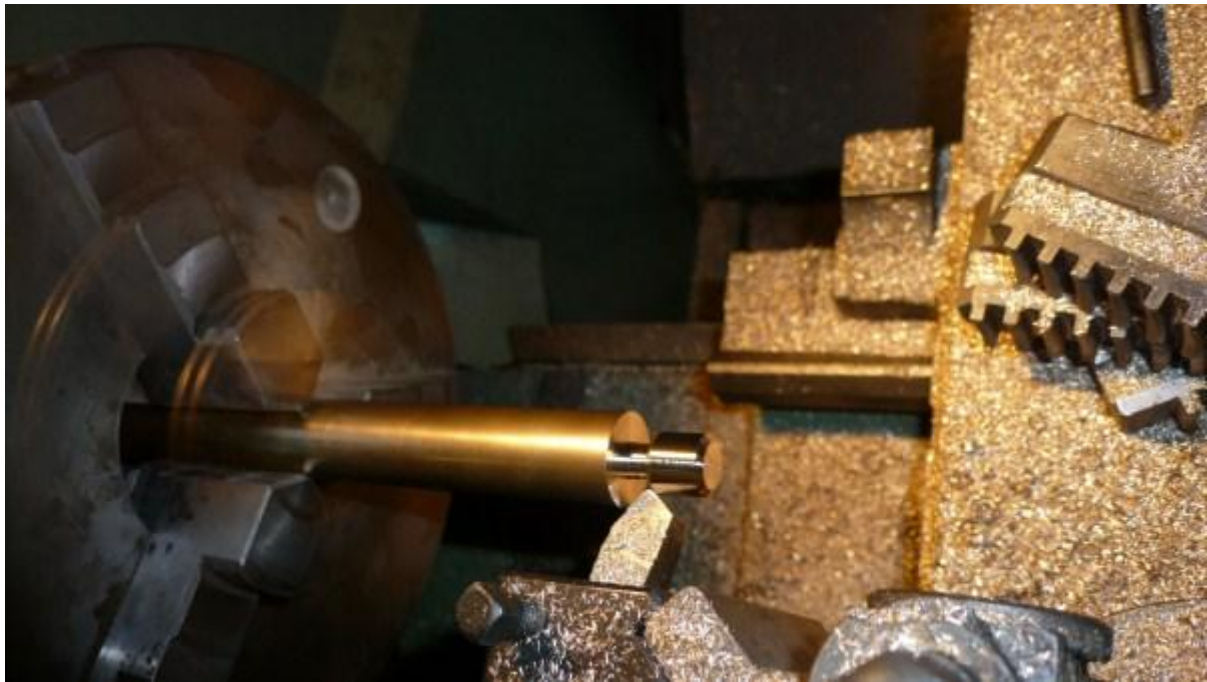
First the rough shape is turned in to the brass stock and the edges chamfered.
