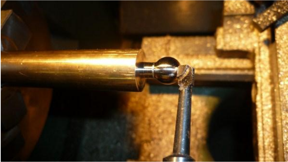
Showing a finishing cut to a ball.
