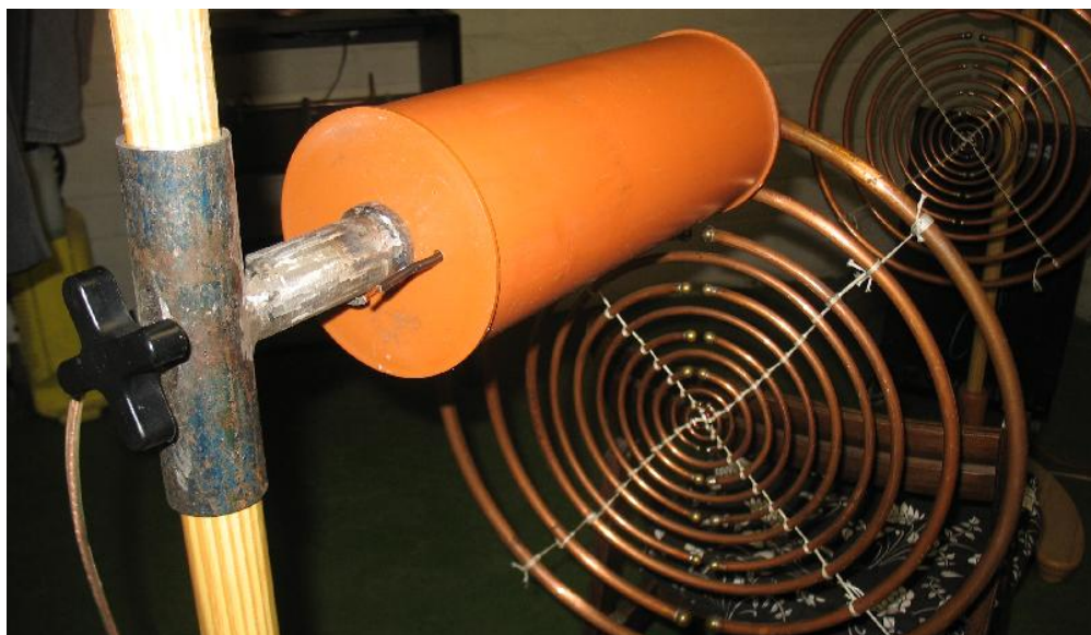
Connection of Tesla coil to antenna holder
