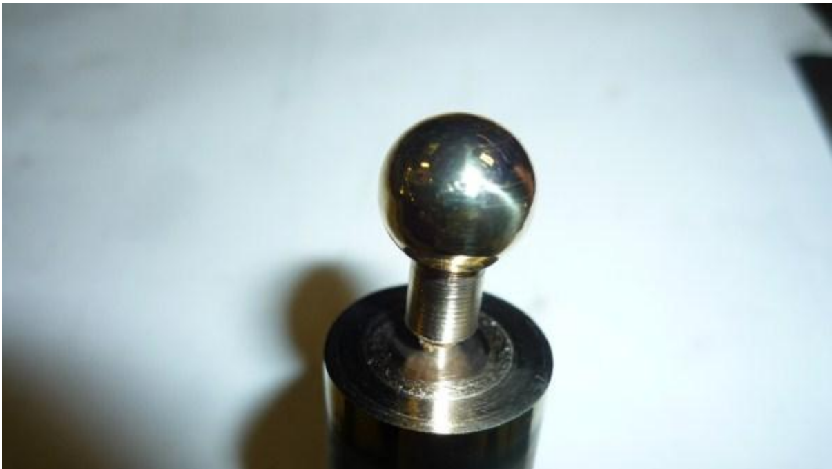
Then while still attached to the brass stock, the ball was polished to final diameter. The shank of the ball was sized to be a tight sliding fit inside the copper tubing.
