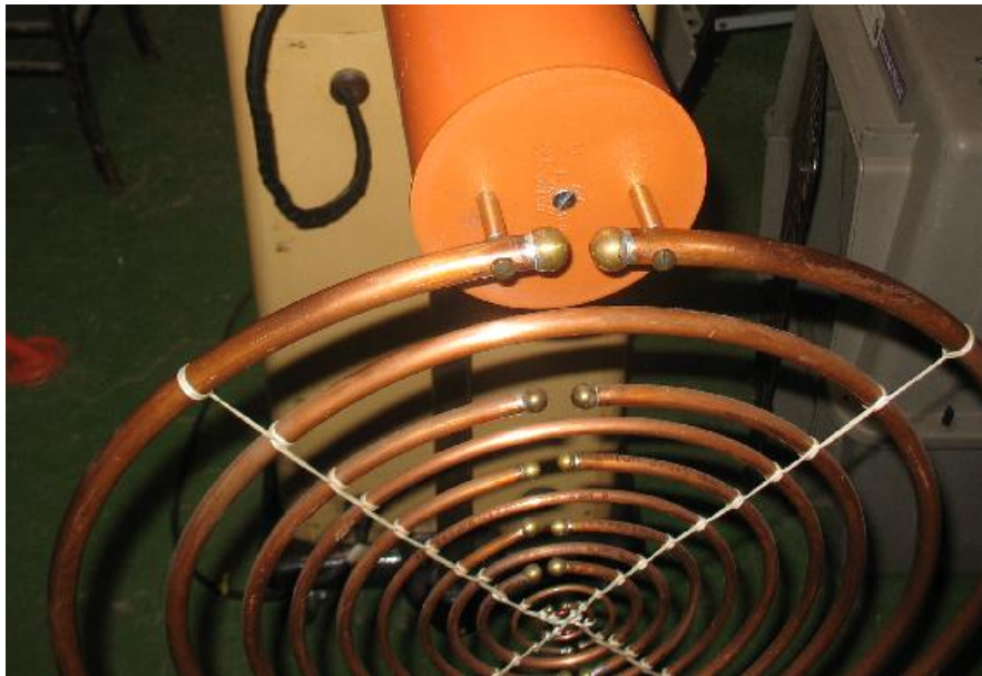
Connection of antennas to the Tesla coils
