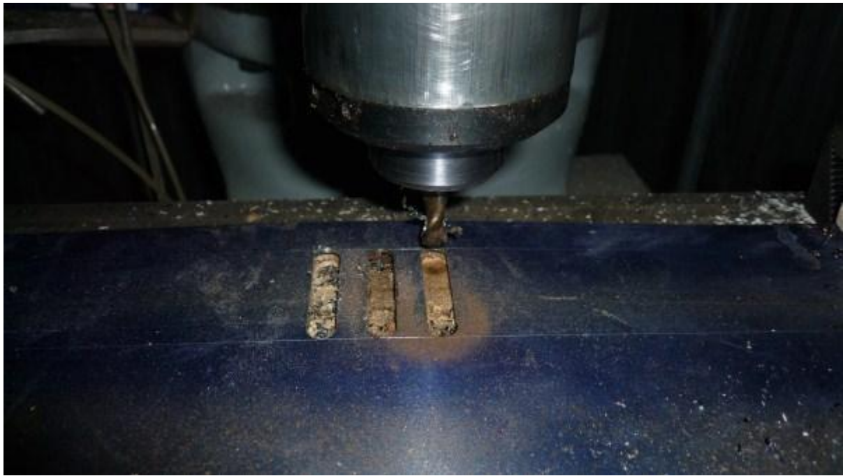
Cooling slots being milled.
